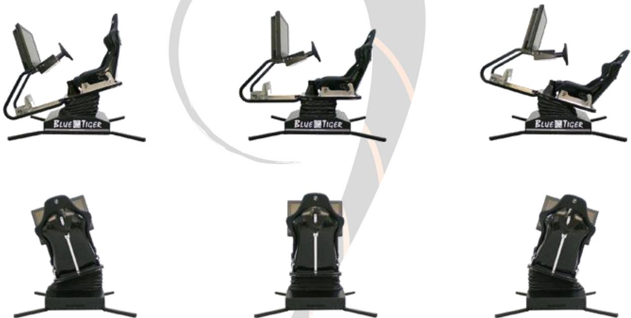
The base of the simulator houses the power supply, control electronics, and motors. The sled is the moving part of the system and is attached to the top of the base. A ballistic nylon bellows is between the base and the sled to protect moving parts from dust and debris. The base uses bolt-on outrigger legs for free standing stability, or it can be bolted directly to the floor (or a floor plate) using flanges.
